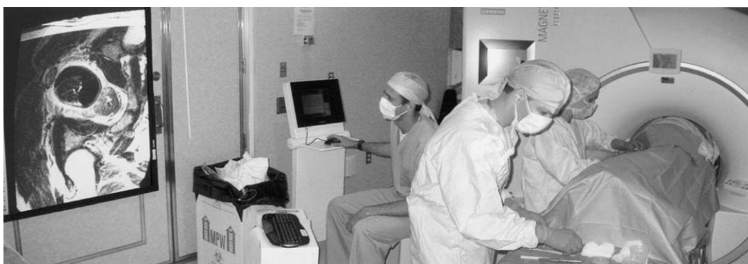
Fig. 2. Magnetic resonance imaging (MRI) scanner room setup. Entire needle placement procedure performed inside of scanner room. Two physicians performed needle placement and one engineer controlled MRI scanner (via in-room console) and targeting and visualization application (via wireless keyboard and mouse). To ease visualization and planning, images were projected onto screen within scanner room.
